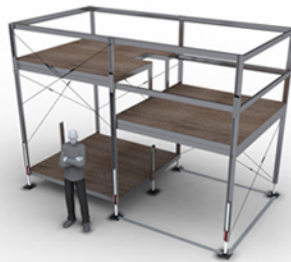
2 assemble frame and floors
